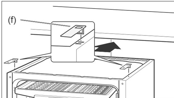
4. Insert the two mounting brackets (f) into the front slots on the top of the dishwasher so that you can screw the dishwasher to the worktop subsequently.
