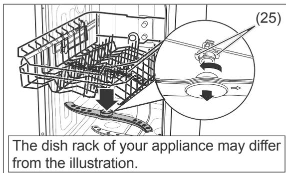
3. The upper spraying arm is affixed using a bayonet closure. To remove the spraying arm, hold the two serrated bayonet grips (25) still and turn the spraying arm clockwise.
