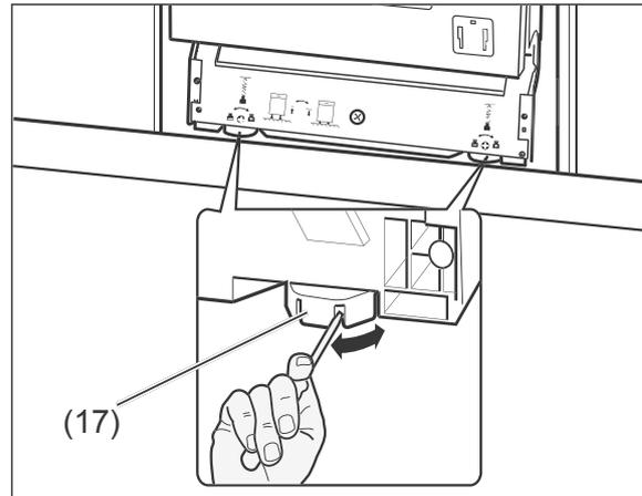
8. To position the dishwasher so that it is level, the two front adjustable feet (17) and the back foot on the appliance can be adjusted by up to 50 mm.
