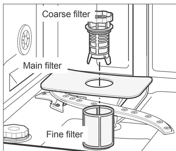
Check the coarse filter, the main filter and the fine filter after each rinse cycle and remove food residues and foreign bodies if necessary:
