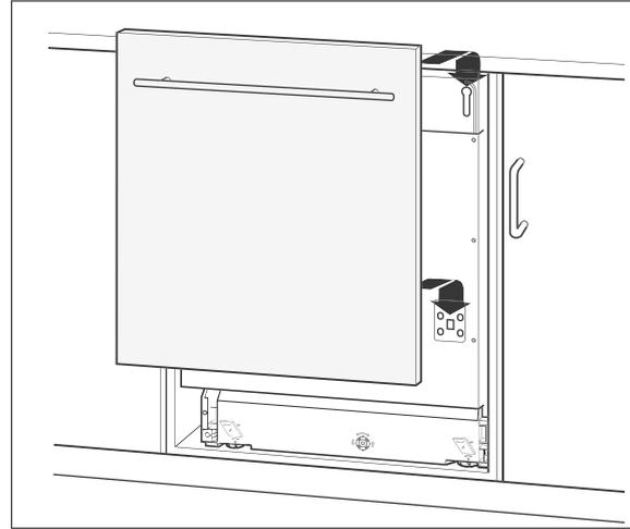
6. Hang the front panel on the appliance door, hold it in place and open the door carefully.
