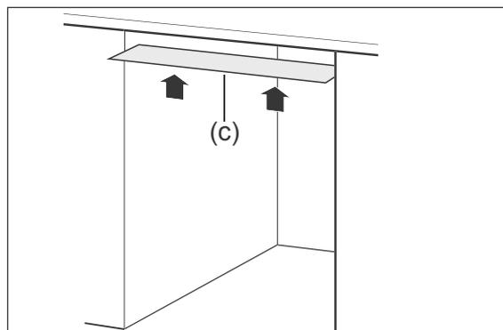
3. Affix the enclosed protective film (c) to the bottom of the work surface. In this way, you will avoid damage to the work surface as a result of hot steam which may be emitted from the dishwasher if the appliance door is left open.
