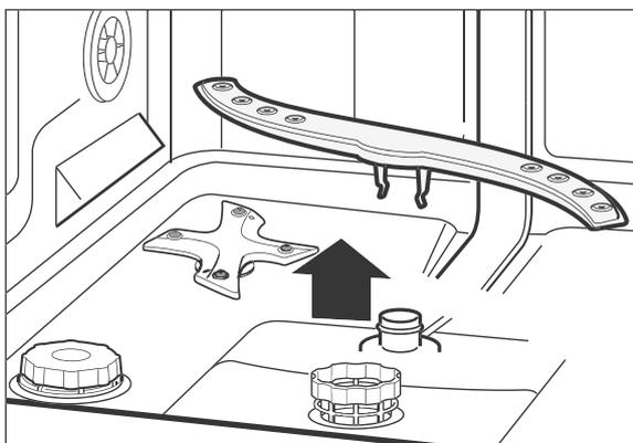
2. Pull the lower spraying arm up and off.
