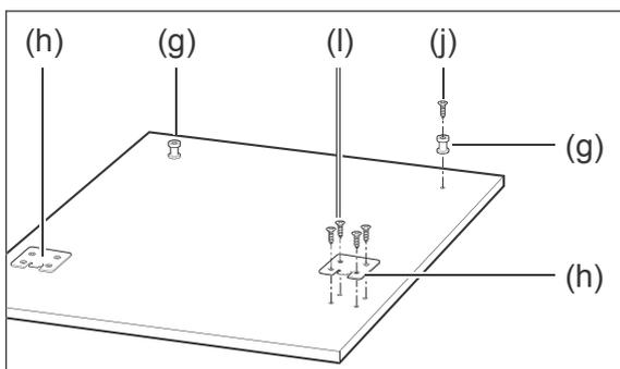
4. Affix both installation hooks (h) with four screws (l) each onto the front panel.
