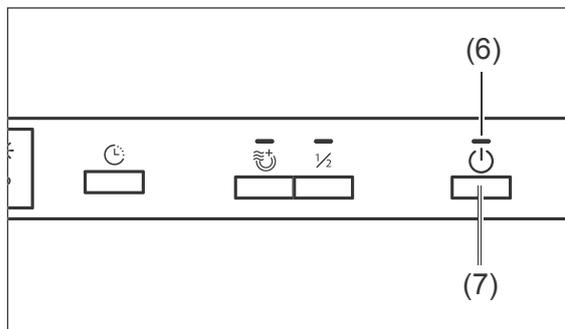
1. Open the appliance door and switch the dishwasher off using the
