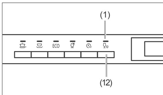
2. Press and hold the
