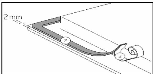
Stick the gasket (2) two millimeters from the external edge of the glass, after removing the protection sheet (3).
