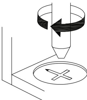
**EN\_**Turn cam lock clockwise to tighten.
