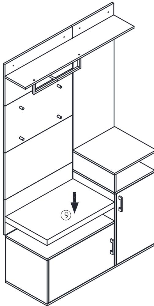
**EN** If it is a solid wall, please use expansion and self-tapping screws, if it is a wooden wall, only use self-tapping screws, please do not overtighten the screws
