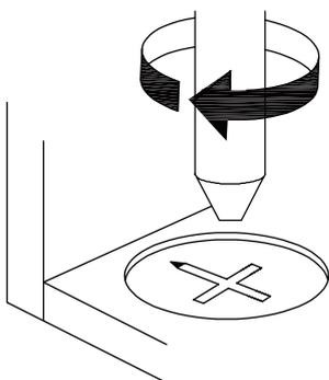
**EN\_**Turn cam lock clockwise to tighten.
