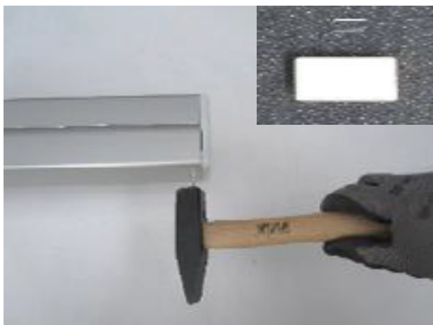
Fixing of cap in square upright
