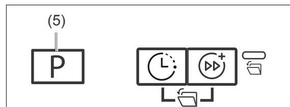
2. Press and hold the **P** button (5) for as long as required until the current water hardness is shown on the display: H 1 to H 6.
