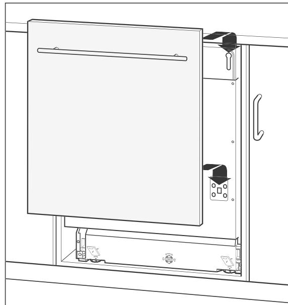
6. Hang the front panel on the door of the dishwasher, hold it in place and open the door carefully.
