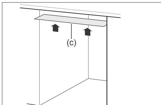
3. Affix the enclosed condensation-protective film (c) to the bottom of the work surface. In this way, you will avoid damage to the work surface as a result of hot steam which may be emitted from the dishwasher door if the dishwasher door is left open.
