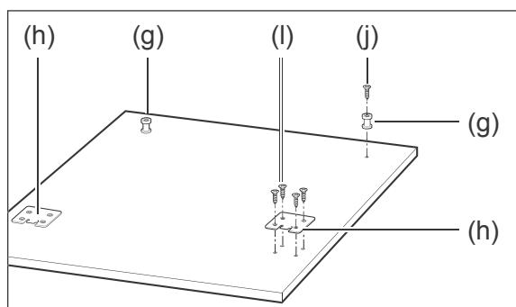
4. Affix both installation hooks (h) with four screws (i) each onto the front panel.
