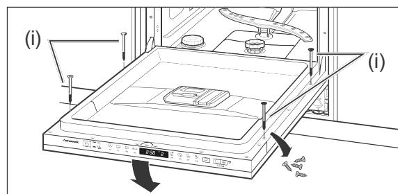
7. Remove the 4 screws from the inside of the door. Screw the front panel in place at these positions using the 4 enclosed screws (i).
