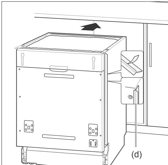
5. Remove the protective films from the side end profiles (d).
