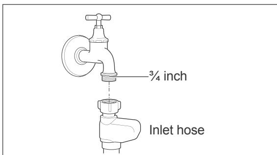
You will require a valve with a  $\frac{3}{4}$ -inch screw connector for the water supply.
