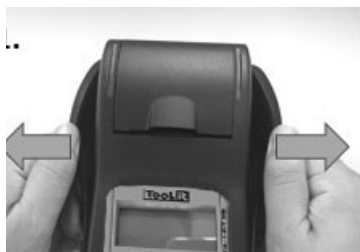
Remove the protective cover
