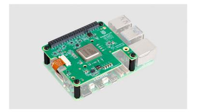
The Raspberry Pi AI HAT+ is an add-on board with a built-in Hailo AI accelerator for Raspberry Pi 5. It provides an accessible, cost-effective, and power-efficient way to integrate high-performance AI. Explore applications including process control, security, home automation, and robotics.
