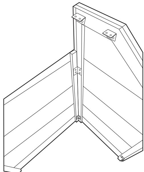
**EN** We will have to unscrew the screws that attach the part "D" to the structure. As it can be seen in the sketch, they are inside the box. Then we remove the piece "D" and we place it in a comfortable place to be able to work on it.
