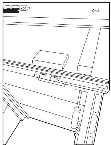
**EN** We will place the new cover "D1" and we will centre it. with the hinges we will make a pre-marking and with the drill bit that comes in the kit we will make some guides for the screws to avoid cracks in the material.
