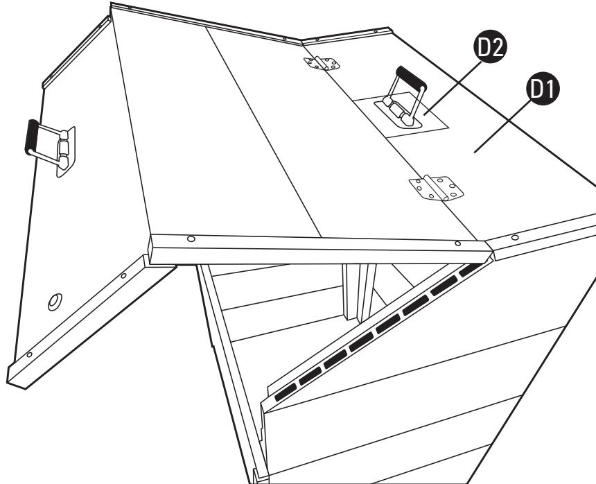
**EN** Finally, we will unscrew the handle of the old lid "D2" and we will screw it on the new one as always, we will centre it, we will make some guides with the drill bit and we will screw the piece.
