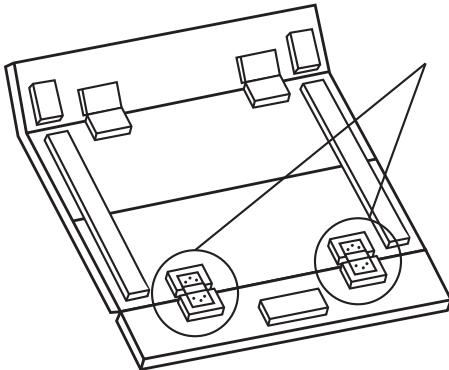
**EN** The next step is to unscrew the 6 screws that are joining the hinge with the upper part of the lid "D1".
