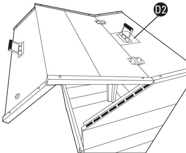
**EN** Now we have to put back the cover "D2" to the structure "D1", we will centre the cover "A" and we will mark the places where the screws have to go and with the drill bit we will make a guide to avoid fracturing the material and we will screw the cover.
