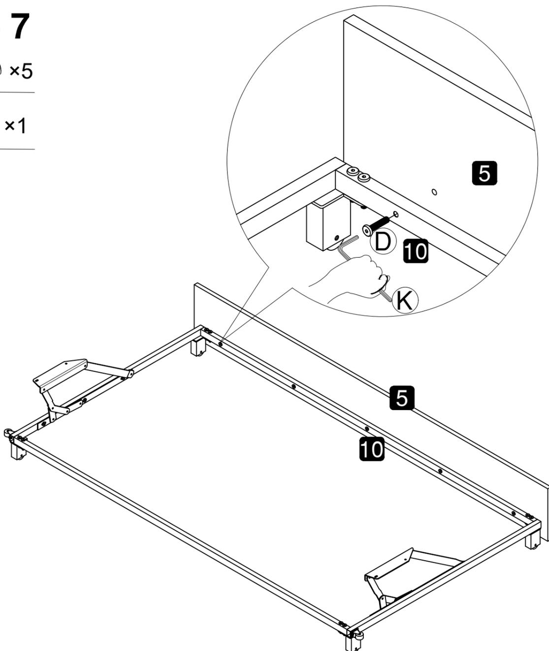
Using an Allen key (K) and bolt (D), connect the Tow bed panel (5) to the Tow bed front tube (10).
