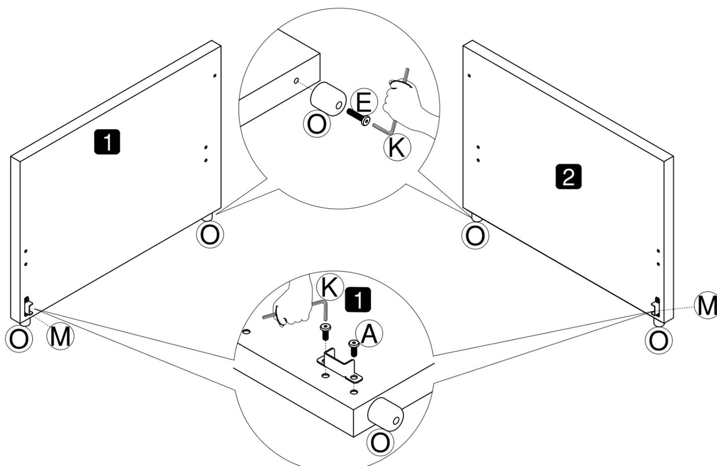
Using an Allen key (K) and bolt (A), secure the Positioning iron sheet (M) to the armrest (1&2), paying attention to the direction, with the opening facing inward.
