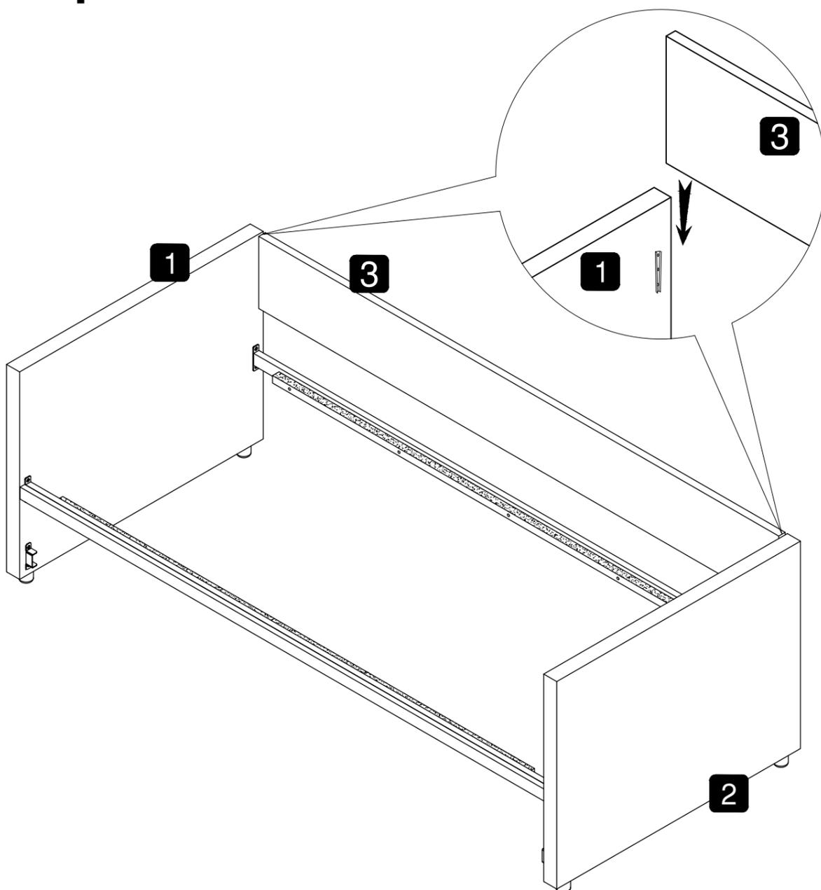
As shown in the figure, hook the backrest (3) onto the armrest (1)&(2).
