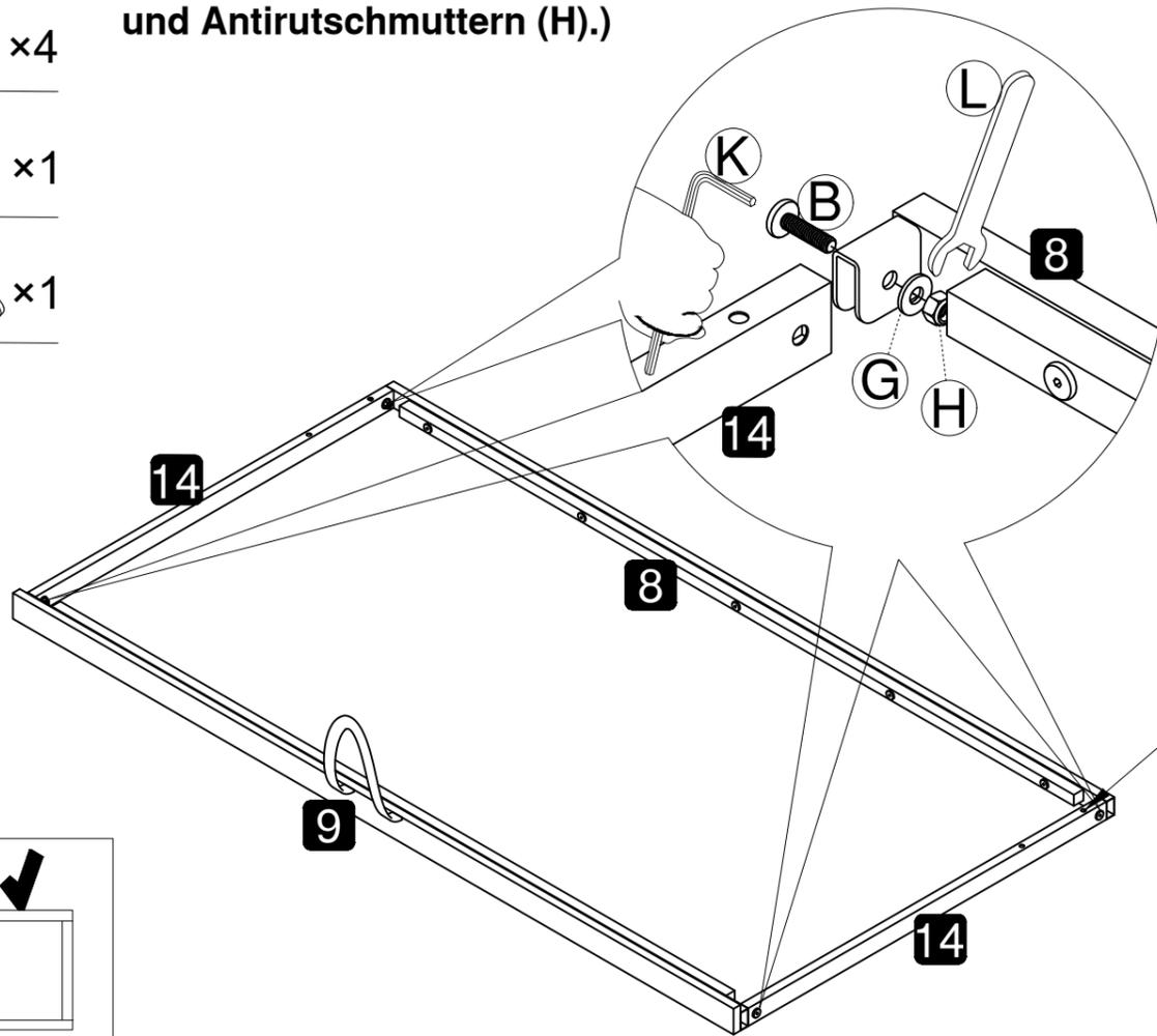
Note the position of the rear bed beam (8) of the traction bed and the front bed beam (9) of the traction bed, as shown in the figure: The rear bed beam (8) of the traction bed is located at the screw hole end of the front tube (14) of the traction bed.
