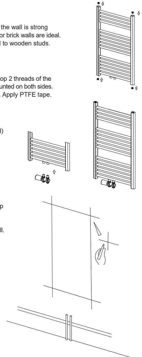
5. Mounting on Brick or Brise Wall Drill the hole with an 8 mm masonry bit at the desired mounting positions and insert the wall plug E into the hole so that it is flush with the wall.
