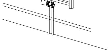
8. Press the rail flat against the wall, adjust to the desired depth and tighten the small screws, slide the end caps over the bracket heads until they lock into place.
