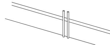
7. Insert the ladder rail A up to the fastening angles and insert the bolt J through the bracket bush K.
