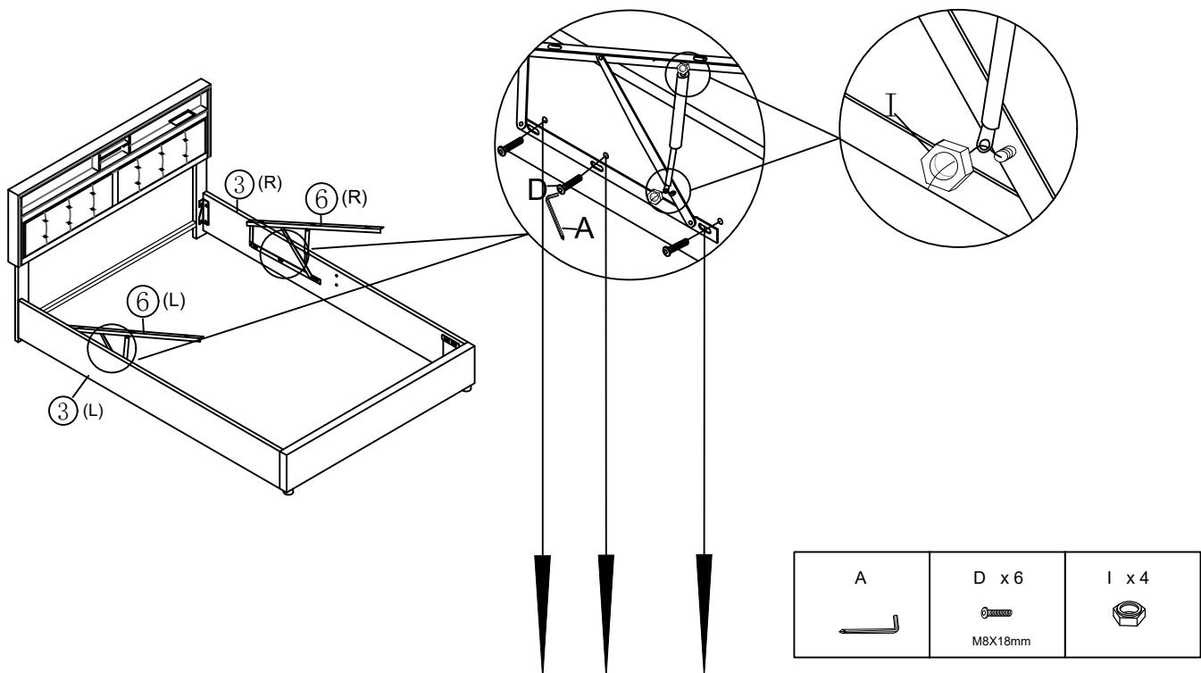
Please note that the hole position here is oval, and the screw can be adjusted back and forth. Please ensure that the position of the left and right bedside hydraulic rods is roughly always.
