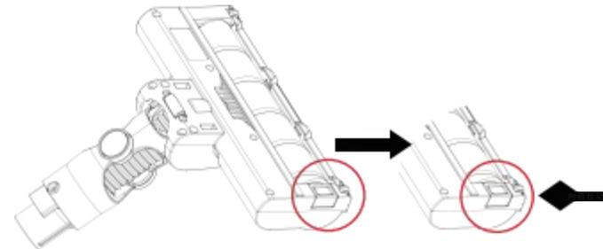
2. Rotate the side part of the floor brush and pull out the roller. (as shown in the picture)
