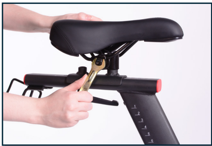
Place seat onto seat post and tighten down and secure with included wrench.
