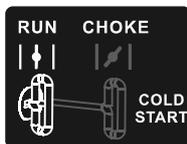
The choke lever must be set to the CHOKE position during cold starting. To start a warm engine, set the choke lever to RUN.
