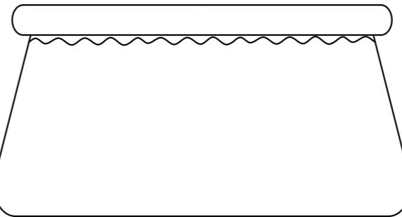
1. Make sure the drain fitting is plugged securely and the cap is in place. Start filling the pool with water. After about 1-inch of water is on the bottom, stop filling and smooth wrinkles out of the bottom of the pool. Pull the outer wall out from the top edge, all around the bottom of the pool, so that it fills evenly.
