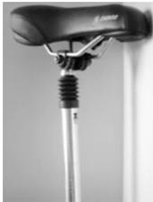
If a suspension seat post is fitted to your bike, the spring comfort can be set using the adjusting nut.
