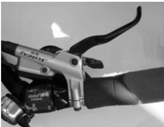
The brake lever is fitted with a supply tank from which brake fluid is pushed to the brake cylinder by pressing on the lever.
