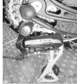
Once free movement is established, the fine adjustments can be made. To do so, shift to 1<sup>st</sup> gear (i.e. the largest cog on the sprocket) and then turn the grip-shift to position 2 for the 2<sup>nd</sup> gear.
