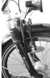
Adjustable suspension forks with lock-out and adjustment
