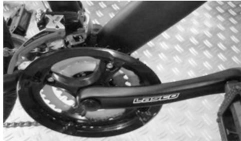
You can work out the number of gears on your bike by multiplying the number of front chain rings by the number of rear cogs, for example 21 gears.
