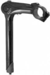
1. Undo the clamping screw under the rubber cover of the stem using a 4 or 5 mm hex key.
