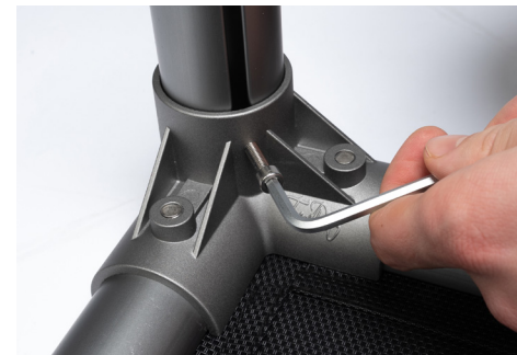
Abb. 6.9.2. Tighten the screw of the legs
