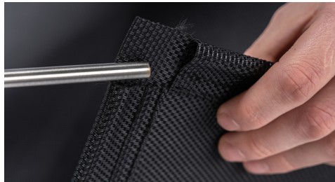
Abb. 6.4.2. Insert the first stainless steel rod into the slot.
