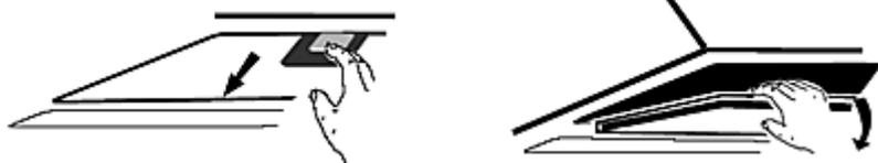
Remove the grease filter(s). The mats are attached to the grease filter or pushed into the sides of the motor.
