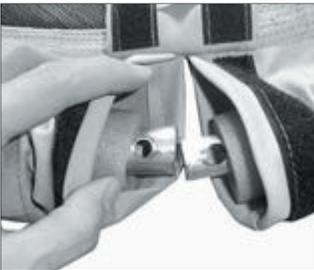
5. Insert the 2nd tube into the sleeve with the small socket inserted into the large socket on the 1st tube.
