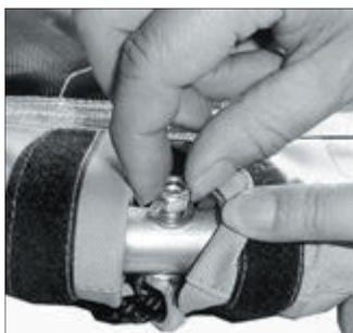
10. Tighten it with a screw nut. Do not forget the washer.
