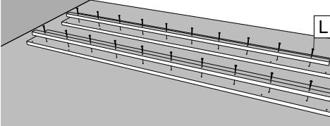
Gently apply pressure on the surface of the panels and secure them with screws.
