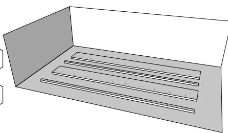
Make sure that left side panel of the bed and right side panel of the bed are clean from dust, dirt and oil.
