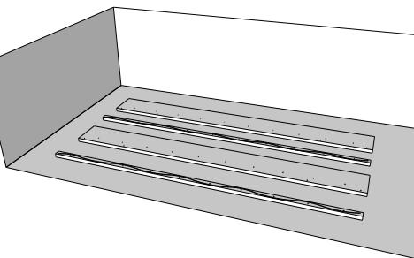
Make sure that all panels that you need to apply glue to are clean from dust,dirt and oil and then apply glue on them.
