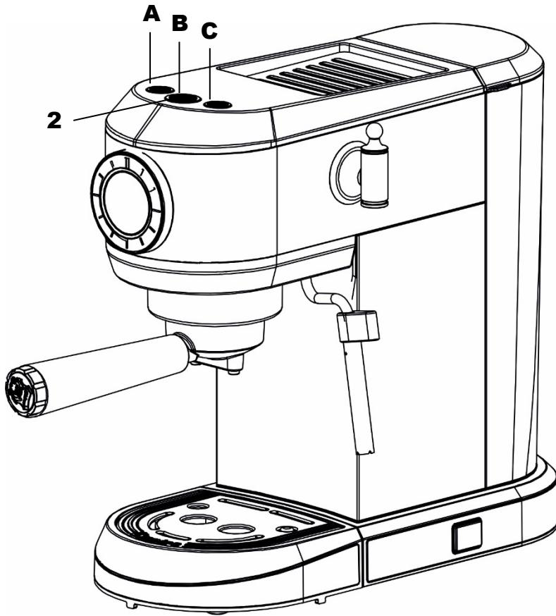
The coffee machine is initially set to use water with a low level of hardness. For your convenience, you can adjust the level of water hardness in your area. In this way, the interval of the descaling operation is increased or decreased.
