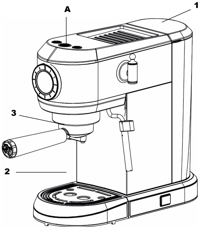
Prepare a descaler. Add it to water tank **1** and fill with 750ml of drinking water. You can find out the ratio of the detergent to water from the manufacturer.
