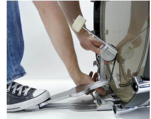
**4.12** Pull the unlocked pedal column (J) a little towards you and take the spring bow (U) off the bearing roll (S). Put the spring bow (U) back on its resting position on the magnet (Z).
