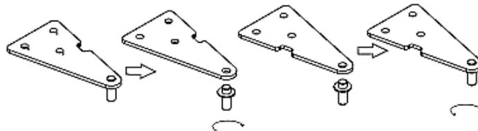
4. Insert the door. Then install the top hinge on the left side. Check that the door is adjusted properly and the door seals close properly before you finally tighten the screws of the top hinge.
