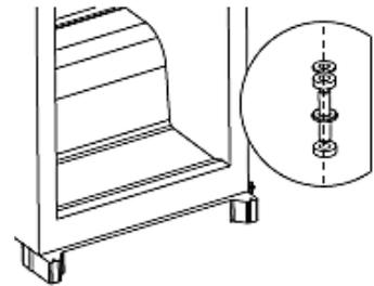
3. Unscrew the top hinge pin. Rotate the hinge and reinstall the hinge pin.
