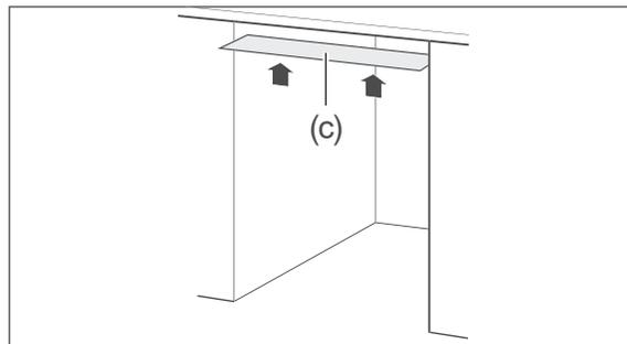
3. Affix the enclosed moisture barrier tape (c) to the underside of the worktop. In this way, you will avoid damage to the work surface as a result of hot steam which may be emitted from the dishwasher if the dishwasher door is left open.
