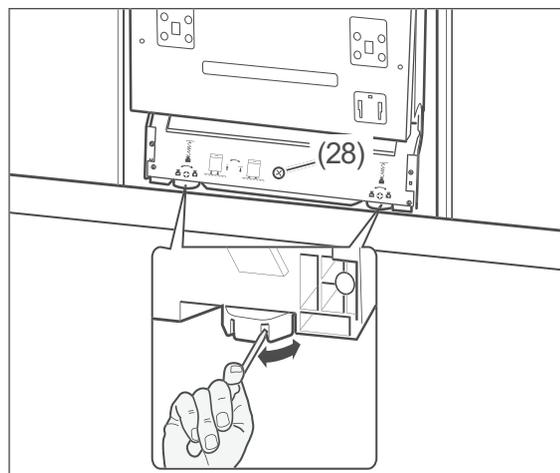
8. To enable the dishwasher to be positioned levelly, both front and back appliance feet can be adjusted by up to 5 cm.
