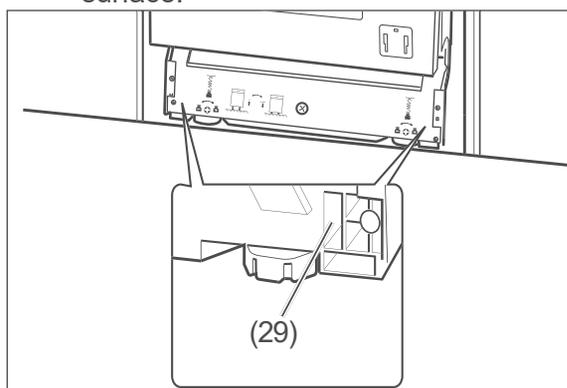
12. If the plinth on your kitchen units is not continuous, you can affix a panel with the help of the plinth holder (o). Plinth holders are screwed to the panel and inserted into the guides (29). To limit the depth, bend out the appropriate slat of the panel holder to the outside.
