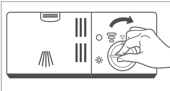
4. Insert the rinse aid dispenser catch (22) and give it a quarter turn clockwise. The markings on the lid and the rinse aid dispenser (22) must be aligned upon insertion.
