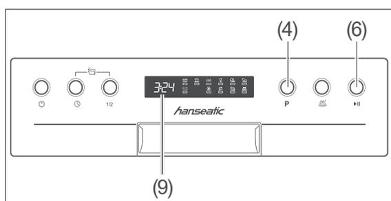
You can interrupt an active dishwashing programme at any point and start a new one. However, do not forget to add extra dishwasher detergent if the programme has already been running for a longer period and the cover of the dishwasher detergent compartment is already open.
