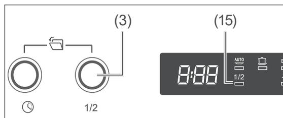
Select the “Half load” option if you would like to run the appliance with less than 6 place settings. This additional option reduces water and power consumption.
