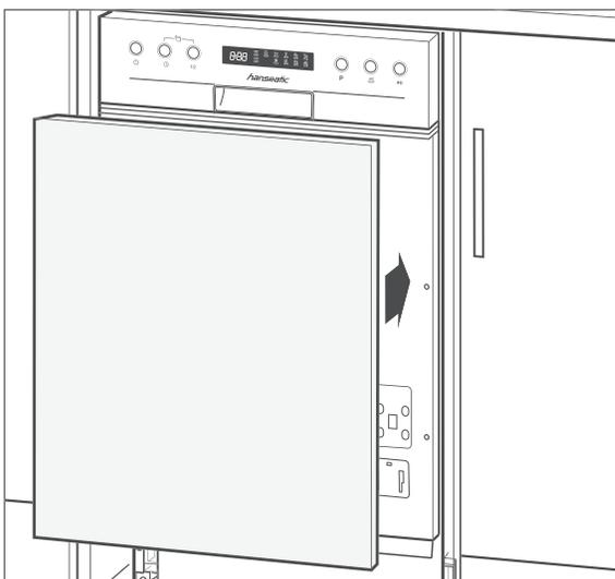
16. Attach the front panel to the door of the dishwasher using the velcro straps (h), hold the panel in place, and carefully open the dishwasher door.
