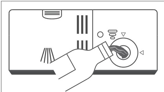
2. Fill the water tank to the "max" mark in the opening. The adjacent inspection window turns black.
