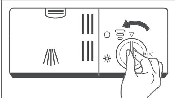
1. Turn the catch of the rinse aid dispenser (22) a quarter turn in an anticlockwise direction and remove it.
