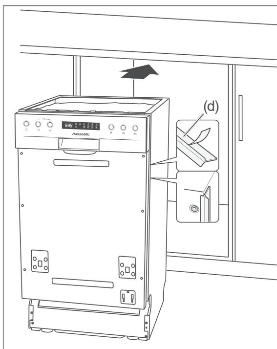
5. Remove the protective films from the side end profiles (d).
