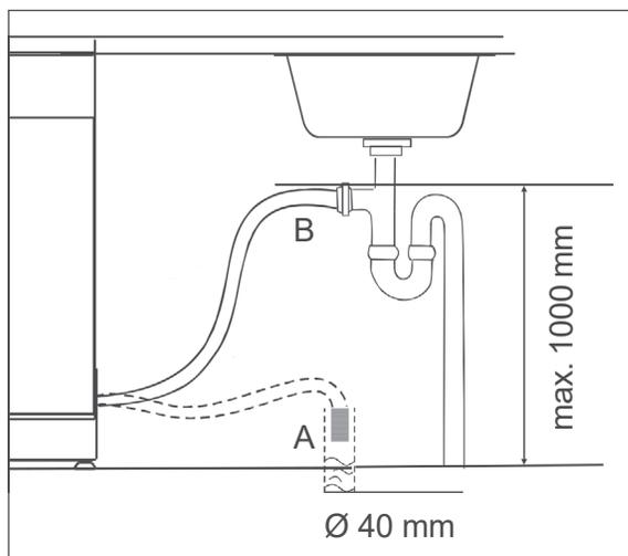
The outlet hose (25) can be connected in two ways:
