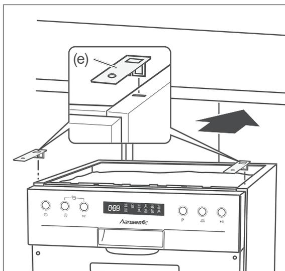
4. Insert the two mounting brackets (e) into the front slots on the top of the dishwasher so that you can screw the dishwasher to the worktop subsequently.
