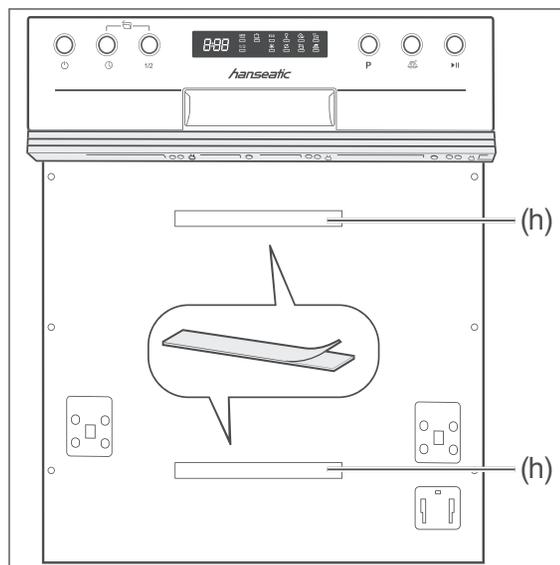
9. With the protective film removed, stick the velcro straps (h) onto the middle of the recessed areas on the dishwasher door.
