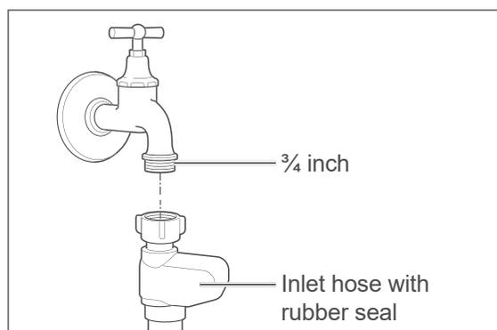
For water supply, you need a water tap with a  $\frac{3}{4}$  inch screw connector.
