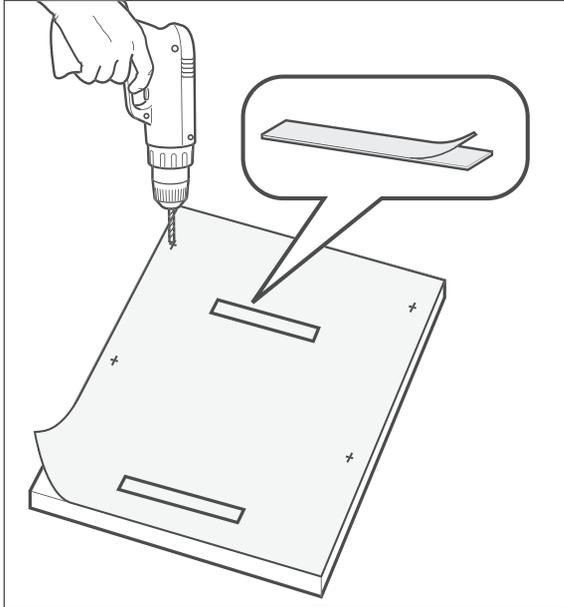
12. Lay the supplied drilling template on the reverse side of the front panel in such a way that the drilling template and the front panel are flush at the top.
