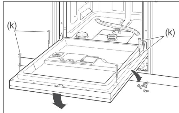
17. Remove the 4 screws from the inside of the dishwasher door. Screw the front panel in place at these positions using the 4 enclosed screws (k).
