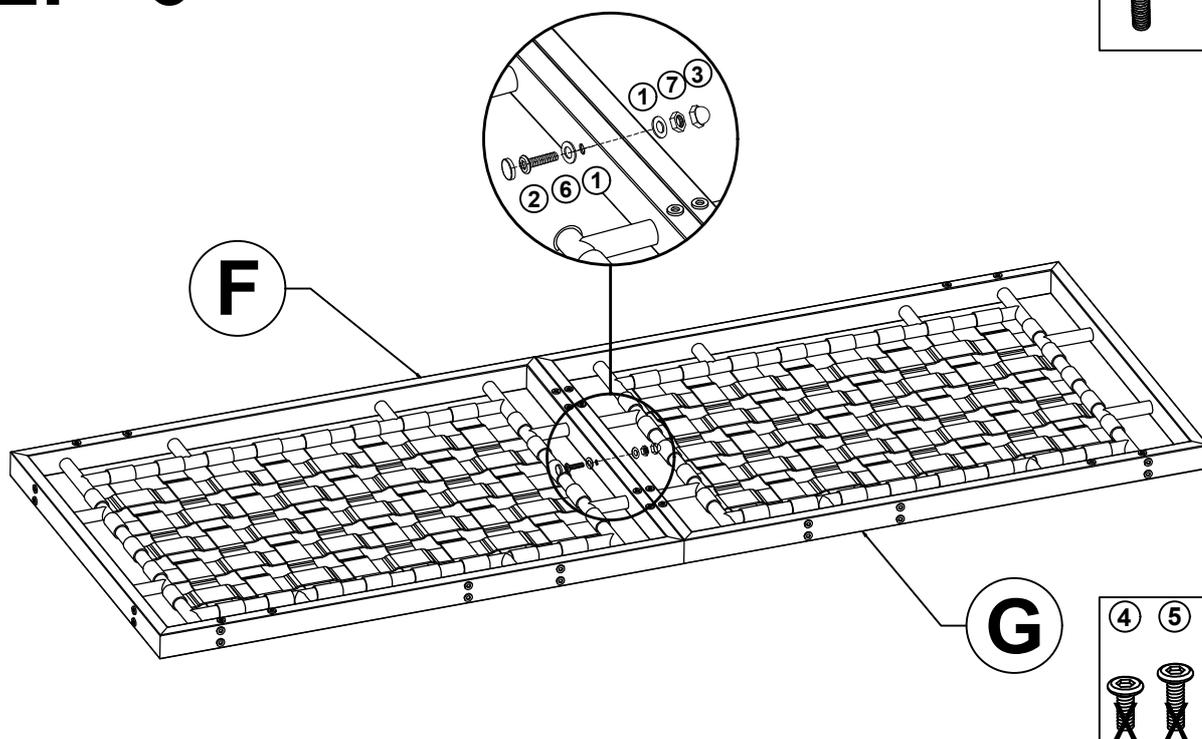
Connect Side Left Bench (F) & Side Left Bench (G) with Bolt (6) & Washers (1) & Nut (7).
