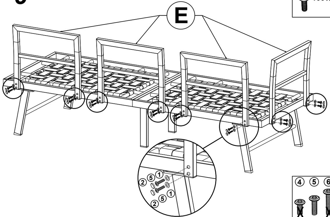
Connect part from Step 8 & Back Frame (E) with Bolt (5) & Washers (1).
