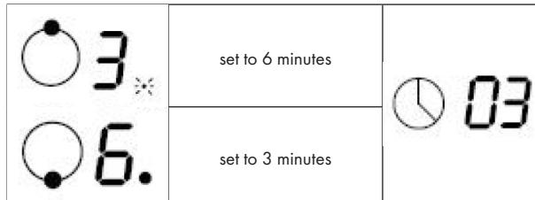
3. When the hob timer expires, the corresponding hob automatically goes off and the screen displays „H“.
