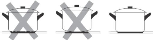
Cookware made from the following materials is not suitable: pure stainless steel, aluminium or copper without a magnetic base, glass, wood, porcelain, ceramic, and earthenware. Do not use cookware with jagged edges or a curved base.
