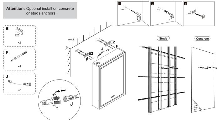
**A** If the cabinet does not fit the wall after the hanger is installed, adjust the two cross screws on the back of the hanger. please refer to last page details.
