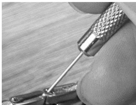
In order to shorten your bracelet to the desired length, you have to remove unneeded connecting pieces. To do this, you need to remove the pins that hold the connectors together. You can recognize this by the small holes on the side.
