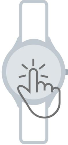
The screen control works by touching the screen with the fingertip and with the two side buttons. Swipe your fingertip to the left or right to get to the watch's various menu options. Press the left button of the watch to return to the main screen. The right button of the watch takes you to the previous screen.
