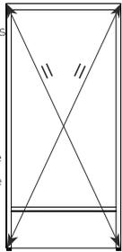
EN- Measure the diagonals of the piece of furniture to check for straightening. The measurement must be identical.
