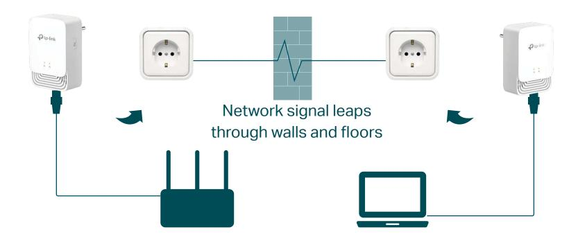
\*G.hn powerline devices are not compatible with HomePlug AV/AV2 powerline devices.
