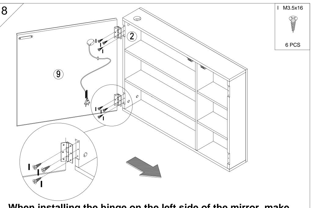
When installing the hinge on the left side of the mirror, make sure the mirror stays flush with the top plate before tightening
