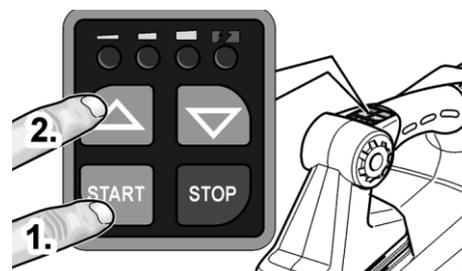
**NOTE:** When operating at maximum speed/Turbo (red LED lights) the blower unit automatically switches a step down after 30 seconds to save battery capacity.
