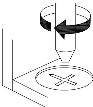
**EN\_**Turn cam lock clockwise to tighten.
