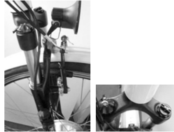
Adjustable suspension forks with lock-out and adjustment
