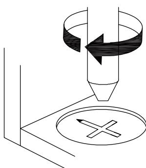
**EN**\_Turn cam lock clockwise to tighten.
