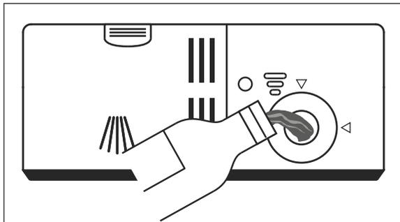
2. Fill the water tank to the "max" mark in the opening. The adjacent inspection window turns black.
