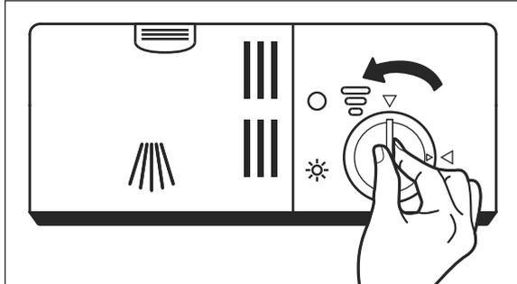
1. Turn the catch of the rinse aid dispenser (19) a quarter turn in an anticlockwise direction and remove it.
