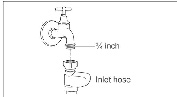
For water supply, you need a water tap with a  $\frac{3}{4}$  inch screw connector.
