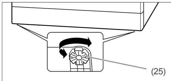
5. In order to compensate for uneven floor surfaces and set up the dishwasher on a level horizontal base, you can screw the four adjustable feet (25) in or out. The adjustable feet have slots around their circumference. Insert a screwdriver and turn the adjustable foot.
