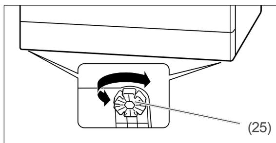
3. In order to compensate for uneven floor surfaces and set up the dishwasher on a level horizontal base, you can screw the four adjustable feet (25) in or out. The adjustable feet have slots around their circumference. Insert a screwdriver and turn the adjustable foot. Use a spirit level to set up the dishwasher.
