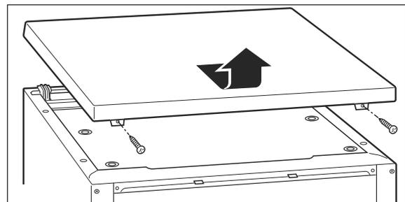
2. Loosen both screws on the reverse side of the covering panel and remove them.
