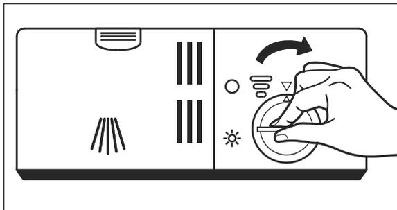
4. Insert the rinse aid dispenser catch (19) and give it a quarter turn clockwise. The markings on the lid and the rinse aid dispenser (19) must be aligned upon insertion.
