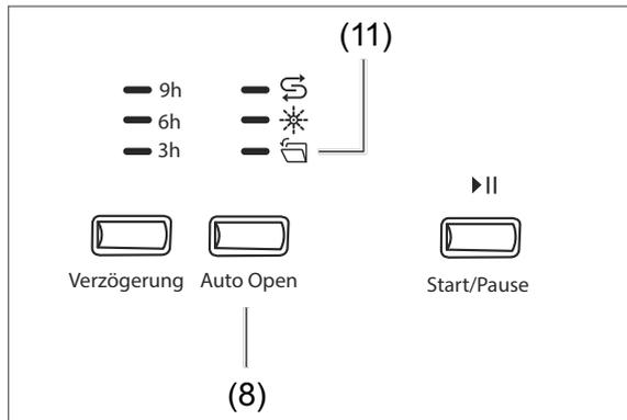
The “Automatic door opening” function is activated as standard.
