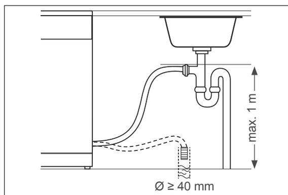
You can connect the end of the outlet hose in two different ways:
