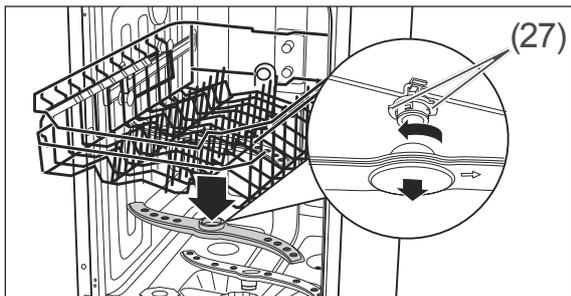
3. The upper spraying arm is affixed using a bayonet closure. To remove the spraying arm, hold the two serrated bayonet grips (27) still and turn the spraying arm clockwise.
