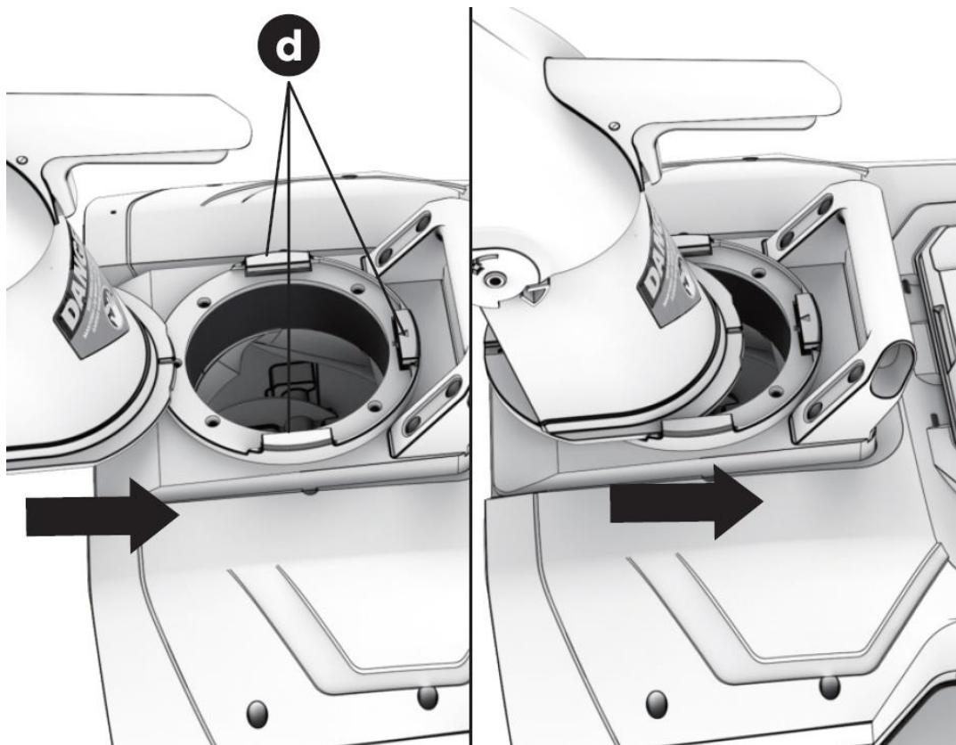
Use a screwdriver (not included in the scope of delivery) to fasten the ejection channel with the supplied screw (see following illustration).
