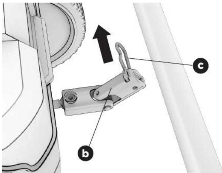
Push the rotary lever of the discharge chute through the holder on the centre handle. Ensure that the crank of the rotary lever is pointing downwards. Then insert the lever into the opening at the rear of the housing. Secure the rotary lever with the split pin (see following illustrations).
