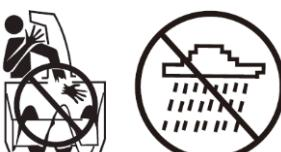
Never reach into the discharge chute while the motor is running!
