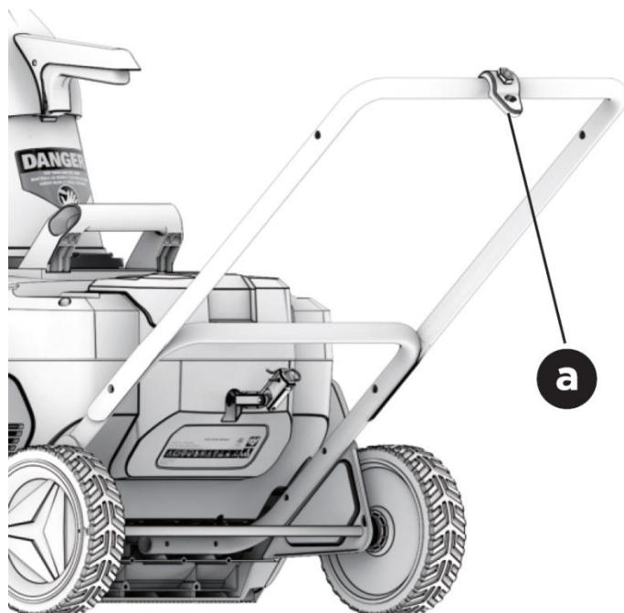
Insert the lever for the bar fixation with washer from the outside of the centre bar through the aligned holes. Attach the connecting piece to the end of the locking lever from the
