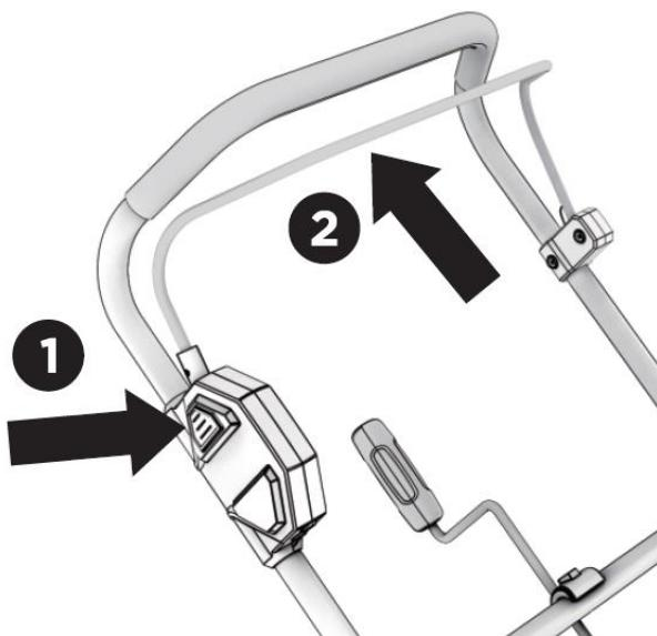
The appliance will now start. When you release the accelerator handle, the appliance stops working.
