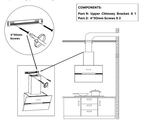
16) Put the Upper Chimney into the Lower Chimney, and then pulled to the height of the Upper Chimney Bracket.
