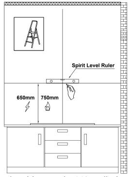
4) Poke the 7 perforated positions on the 1:1 Installation Diagram, then align with the center point of aluminum grease filter on the Installation Diagram with the horizontal line on the wall, then tape the Installation Diagram to the wall, and use a pencil to mark the perforated positions on the wall in the corresponding positions.
