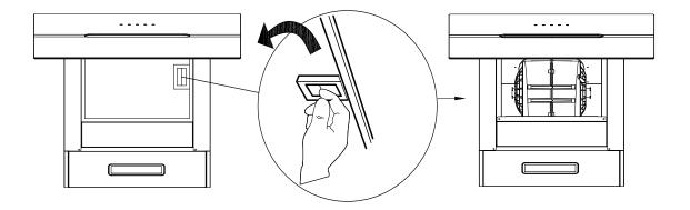
2. Place the carbon filter into the unit and turn it in the clockwise direction to lock it in place.
