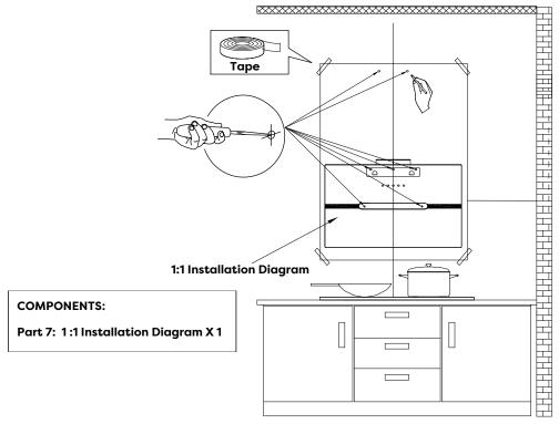
5) Determine the maximum chimney installation height according to the actual scenario and mark the chimney installation locations along the center line of the Installation Diagram.
