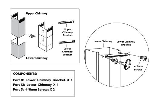
13) Insert the Lower Chimney into the hood and fix it to the corresponding positioning hole with two 4\*8mm Screws. (Note: That the power cord needs to go through the chimney and connect the power).
