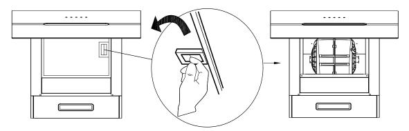
2. Push the LED lamp holder out from the cabinet by hand, or use screwdriver to prize up the LED lamp around the edges, pull out slotted the LED lamp and the wire together.
