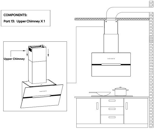
17) Use two 4\*8mm Screws to assemble the Upper Chimney on the Upper Chimney Bracket.
