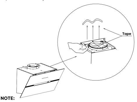
Make sure you remove the tape on the damper and check if the damper opens and closes freely, otherwise it make noises, and the cooker hood will be shaking.
