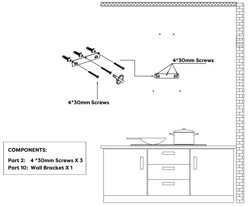
8) Remove the aluminum grease filter and hang the hood on the corresponding hook of the Wall Bracket.
