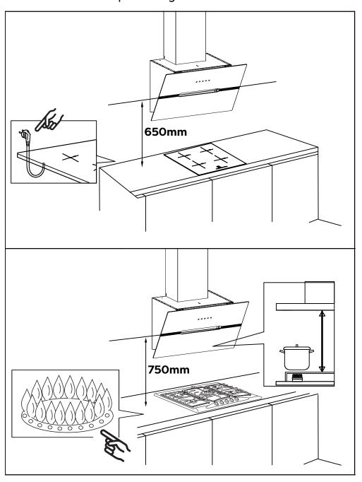
3) First use a pencil to mark the installation position on the wall, then use a Measuring Tape to measure the height from the stove surface to the hood (the center point of aluminum grease filter) and use a Spirit Level Ruler to maintain the level, then use a pencil to draw a horizontal line along the level.
