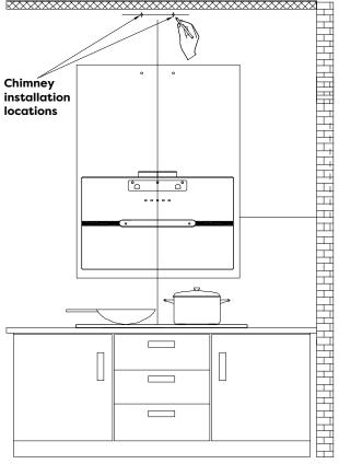
6) Remove the Installation Diagram, drill the holes that have been marked on the wall with an Electric Drill (8mm drill), and hammer the Wall Plug into the wall.
