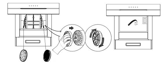
3. If the carbon filter needs to be replaced, please turn it in the anticlockwise direction.
