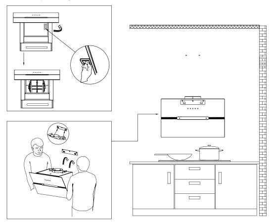
9) Use a Spirit Level Ruler to measure whether the hood is in a horizontal level, and use two 4\*30mm Screws to lock into the safety hole position of the hood (not mandatory, according to user's wishes to choose whether to lock).
