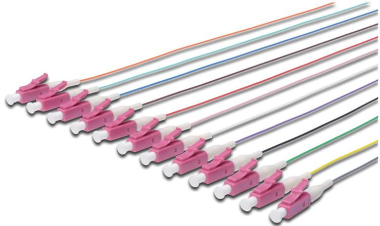
**LWL Pigtail-Set, 12 Stk., LC, MM OM4 50/125 µ loose buffer, Farbcode DIN IEC 304, 2 m**
