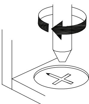
**EN**\_ Turn cam lock clockwise to tighten.
