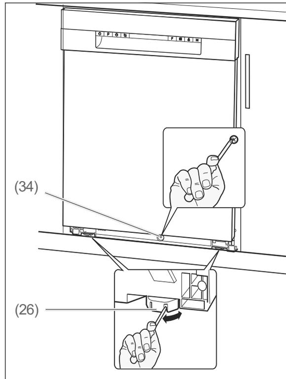
1. Insert a crosshead screwdriver into one of the slots and turn the adjustable feet (26) to the height required.
