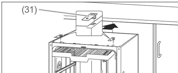
4. Insert the two mounting brackets (31) into the front slots on the top of the appliance so that you can screw the appliance to the worktop later on.
