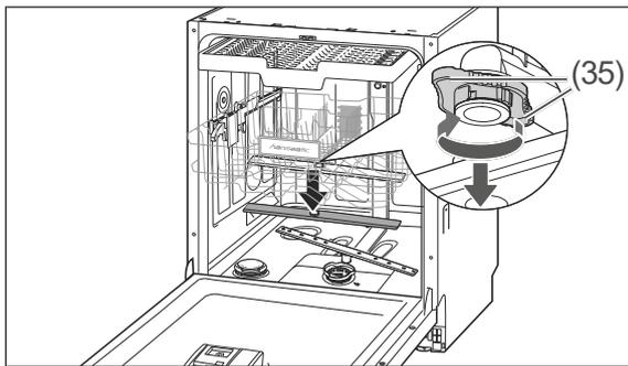
3. The upper spraying arm is affixed using a bayonet closure. To remove the spraying arm, hold the two serrated bayonet grips (35) still and turn the spraying arm clockwise.
