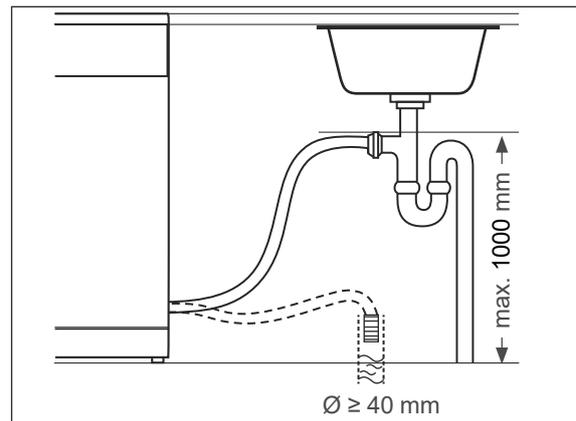
You can connect the end of the outlet hose (15) in two different ways:
