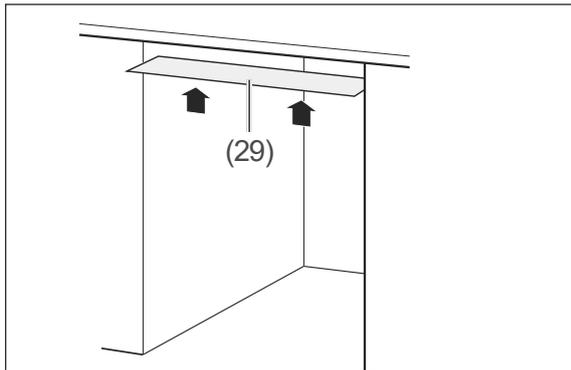
3. Affix the condensation protection film supplied (29) to the underside of the work surface. This will prevent damage to the worktop caused by hot steam released from inside the dishwasher when the appliance door is left open.
