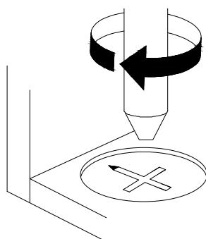
EN Turn cam lock clockwise to tighten.
