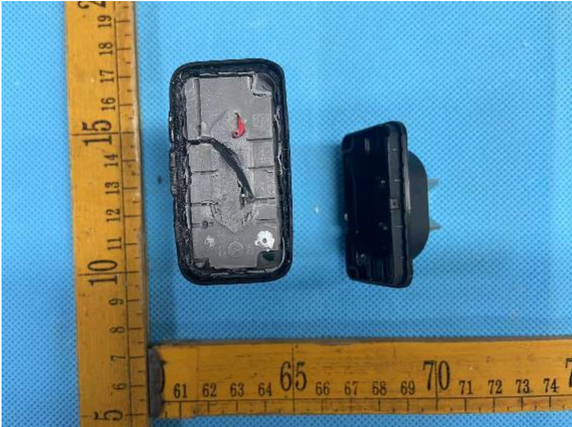
Picture 17. Internal view (AU plug)
