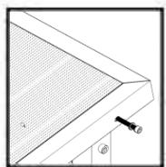
Turn the roof over so that the flat side is on top. Using two people, lift the roof onto the shelf and connect it to the frame at the corners using the screws (B). Now tighten all the screw connections of the shelf. Carry the shelf to its destination in pairs. Make sure that the surface is level and that the feet are all on the same level.
