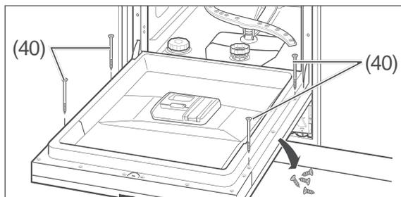
7. Remove the 4 screws from the inside of the door. Screw the front panel in place at these positions using the 4 enclosed screws (40).
