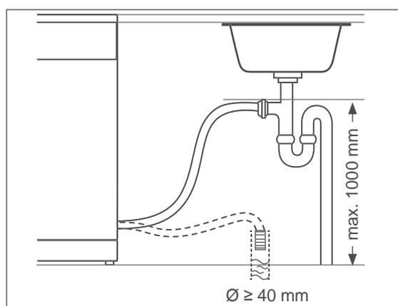
You can connect the end of the outlet hose (19) in two different ways:
