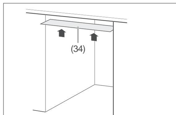
3. Affix the enclosed condensation-protective film (34) to the bottom of the work surface. In this way, you will avoid damage to the worktop as a result of hot steam which may be emitted from the interior if the door is left open.
