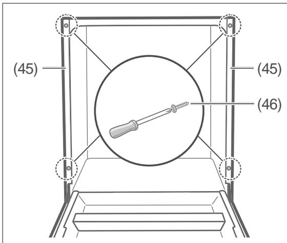
5. Remove the four side strip screws (46) from the side strips (45).
