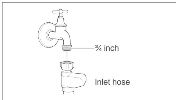
You will require a valve with a 3/4-inch screw connector for the water supply.
