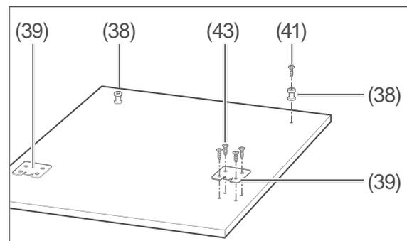
4. Affix both installation hooks (39) with four screws (43) each onto the front panel.
