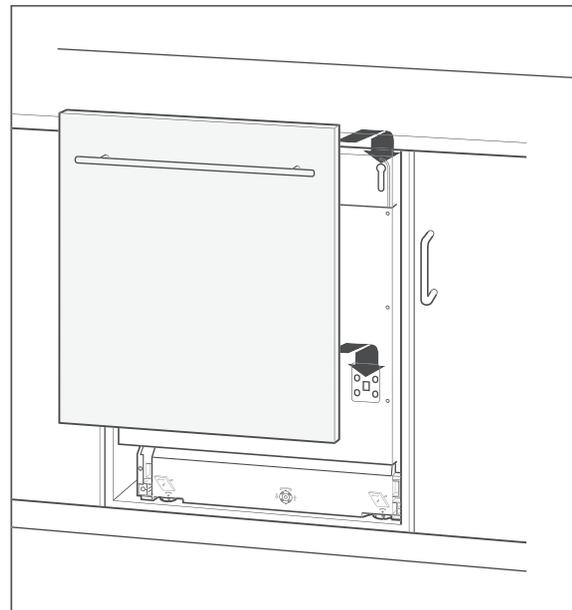
6. Hang the furniture front panel on the appliance door, hold it firmly and carefully open the appliance door.
