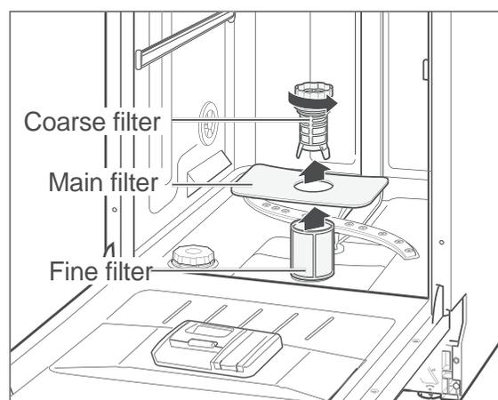
Check the coarse filter, the main filter and the fine filter after each rinse cycle and remove food residues and foreign bodies if necessary:
