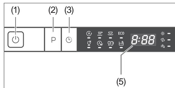
3. Press the **P** button (2) for 5 seconds within 60 seconds of switching on.
