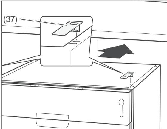
4. Insert the two mounting brackets (37) into the front slots on the top of the appliance so that you can screw the appliance to the worktop later on.
