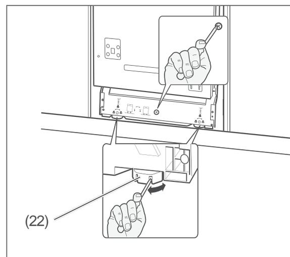
1. Insert a crosshead screwdriver into one of the slots and turn the adjustable feet to the height required.
