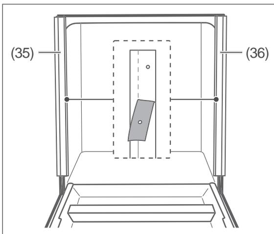
6. Remove the protective films from the left insulation strip (35) and the right insulation strip (36).
