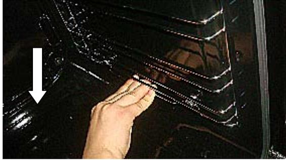
2. Pull the detached side rack forward slightly (s. fig. below).
