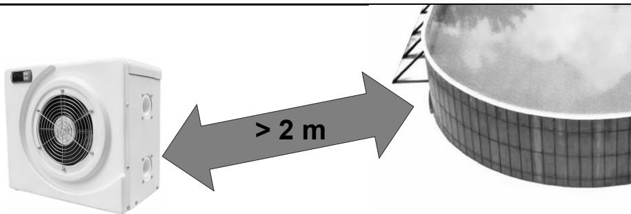
Install the pool heat pump on a flat, horizontal, and stable surface. (Concrete base would be ideal).
