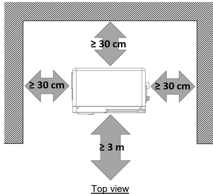
Make sure that the discharged air will not be sucked back into the evaporator again.
