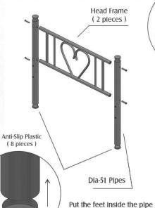
Step 2 Head Side And Back Rail Traverse Assembly
