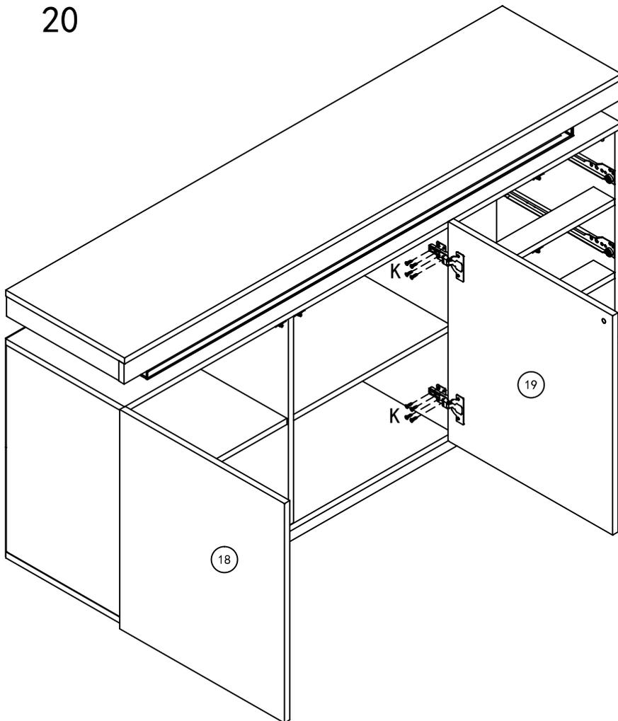
When the hinges are installed, you can refer to the pictures to adjust crevice of the doors till it's perfect:
